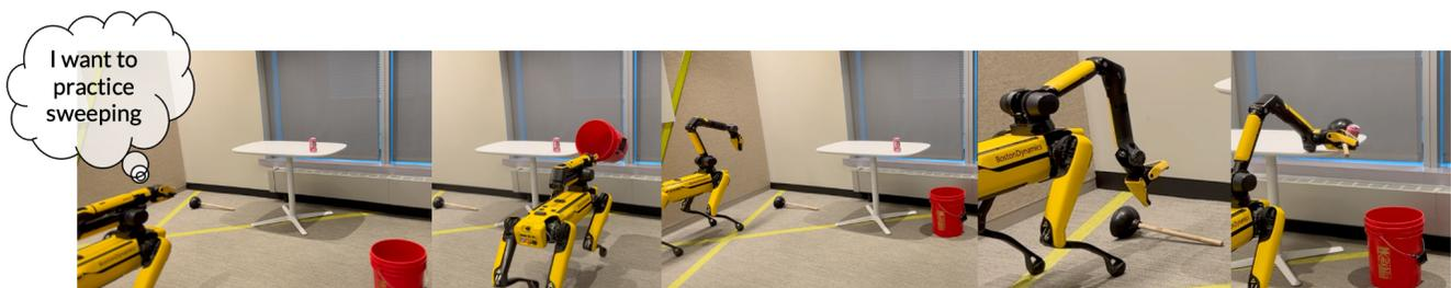
**Figure 1:** Planning to learn. The robot decides what to practice (sweeping with a plunger) and how to practice it (continuous parameters). It then uses planning to autonomously set up a scene where sweeping is possible.
